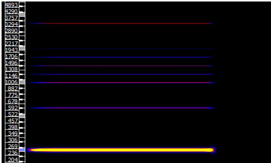
**Fig. 6.** Spectrogram of the timbre generated by the *Pure Data* patch, done with Sonic Visualiser. The horizontal axis represents time and the vertical, frequency channels. Notice the different partials' amplitudes encoded in color difference.
